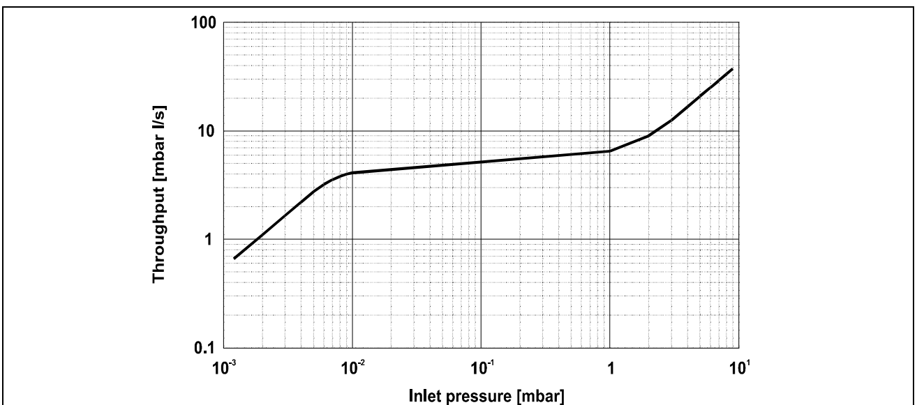
Graph of nitrogen throughput vs inlet pressure using the recommended mechanical forevacuum pump
